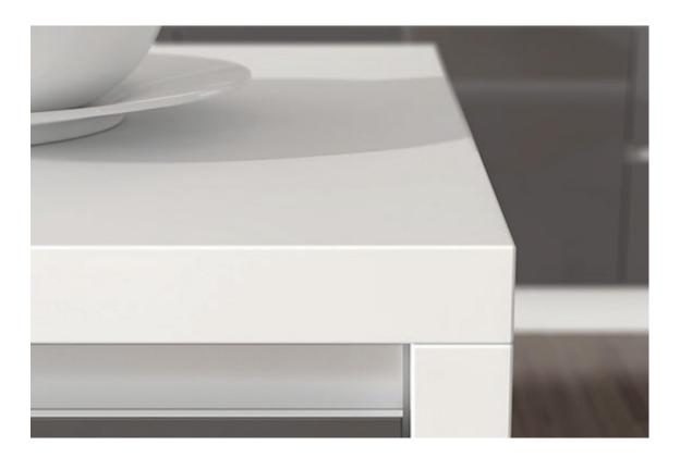
The highlights of ZOW 2014 for the worktop specialist Danielmeyer included the "laser edge". The edges are finished entirely without glue. As a result and especially in the case of white decorative finishes this produces a visual and functional zero joint between the top and the edge. The result is high-quality aesthetics as if made from one piece that offers completely new creative approaches and variations in kitchen design.
